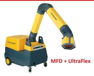
The MFD is a mobile welding fume filter with integrated fan for regular welding applications. It contains an aluminium spark arrester and a disposable filter cartridge. A filter pollution indicator indicates when filter replacement is required.
